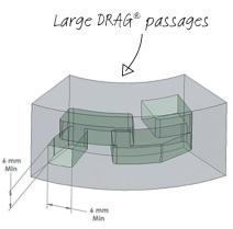
Each right angle turn is a single stage of pressure drop. Large expanding DRAG® flow passages enable sand and paraffin to pass through the trim
