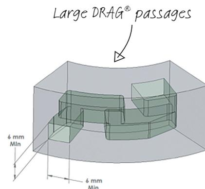
Each right angle turn is a single stage of pressure drop. Large expanding DRAG® flow passages enable sand and paraffin to pass through the trim
